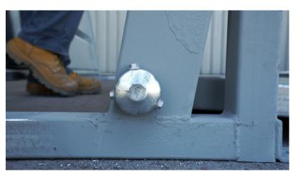
Installing the Slam Latches, locate a spring, shaft and handle. Place the spring inside the hole first followed by the shaft.
